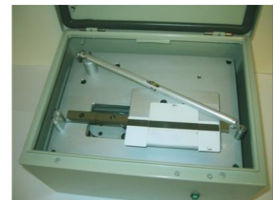
Test Head moved aside for card loading
