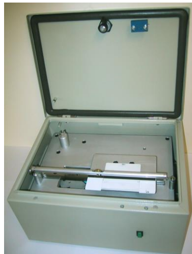
General view. Card loaded for test ISO/IEC Test Head carried in load arm
