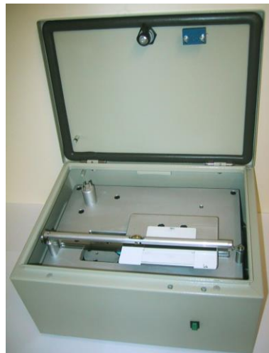
General view. Card loaded for test ISO/IEC Test Head carried in load arm
